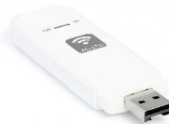
The CANedge2 can also connect to a 3G/4G USB router to upload on-the-road. The hotspot can optionally be powered via the device
