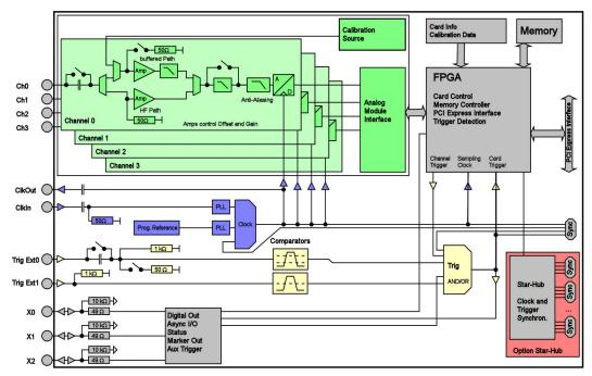
Block diagram of Digitizer Module inside hybridNETBOX DN2.82x
