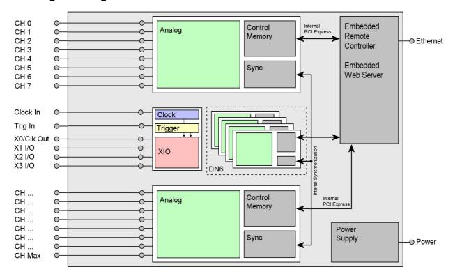
• The number of maximum channels and internal digitizer modules and existance of a synchronization Star-Hub is model dependent.
