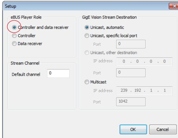
4. Under **GigE Vision Stream Destination**, click **Multicast** and enter the IP address and port number. The address and port must be identical to that configured for the vDisplay HDI-Pro External Frame Grabber in step 8 and 9 of [“To configure the vDisplay HDI-Pro External Frame Grabber for a multicast network configuration”](#) on page 64.
