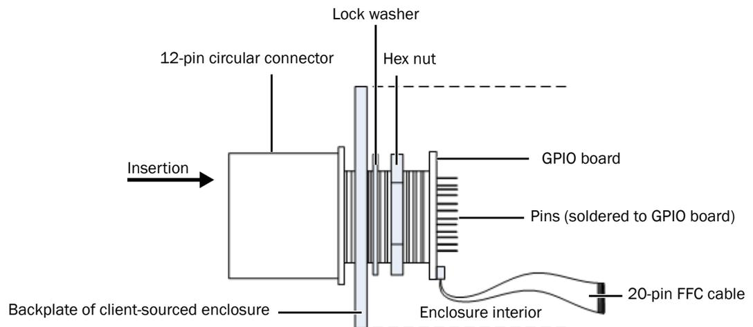
4. Assemble the 12-pin power, GPIO, and serial circular connector to the GPIO board by lining up the pins with the GPIO board.
