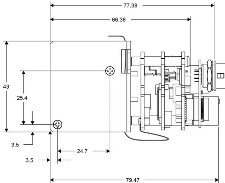
Figure 5: SB-GigE-EV7520A GigE PHY Board Front with Dimensions
