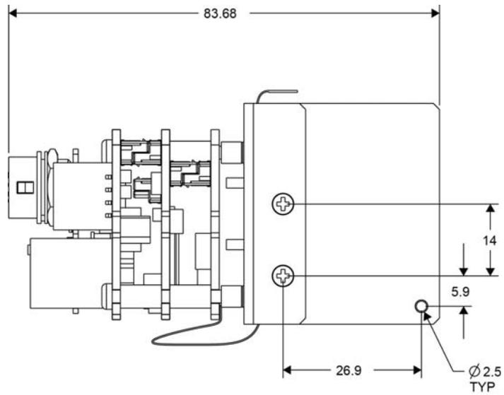
Figure 7: SB-GigE-EV7520A with Brackets Top View
