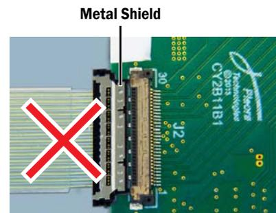
**INCORRECT** when the metal shield on the cable connector is visible.
