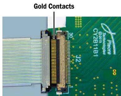
**CORRECT** when the gold contacts on the cable connector are visible.
