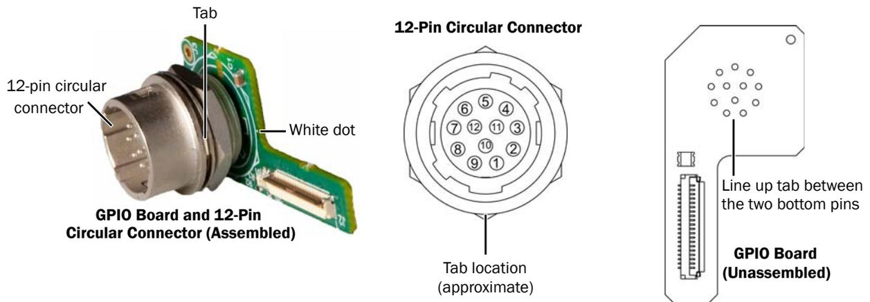
5. Solder the pins of the connector to the GPIO board for a secure connection.
