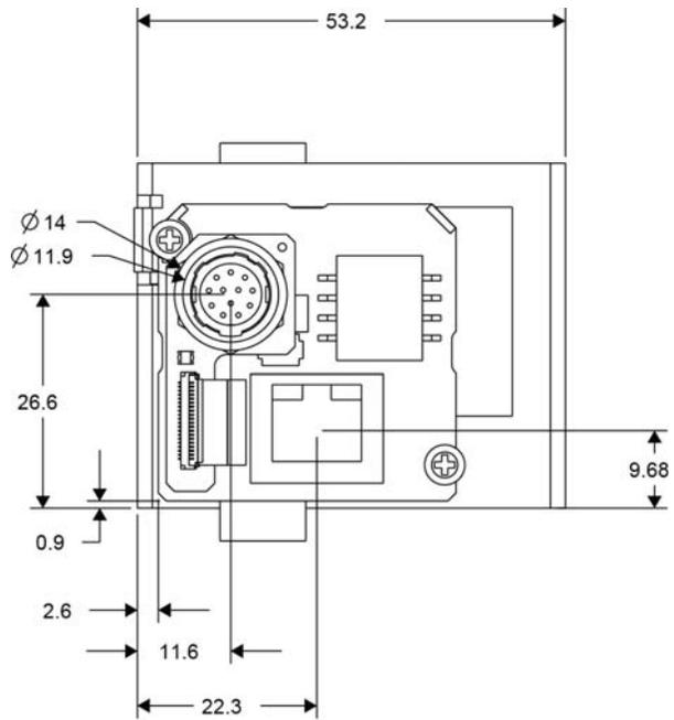
Figure 6: SB-GigE-EV7520A with Bracket Mounting Screw Dimensions
