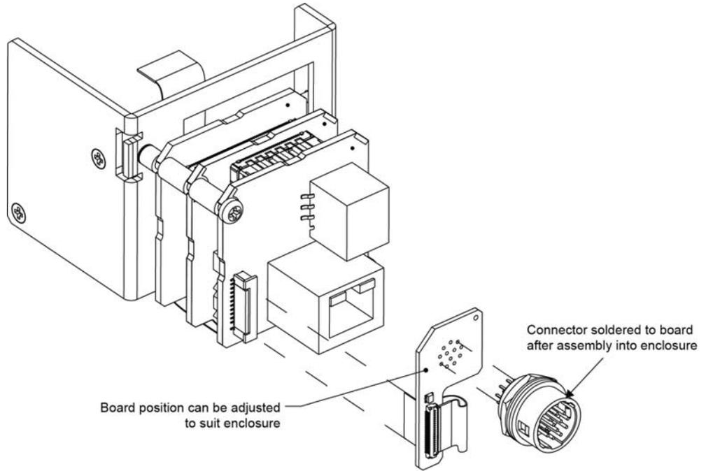
Figure 8: SB-GigE-EV7520A with Brackets Top View
