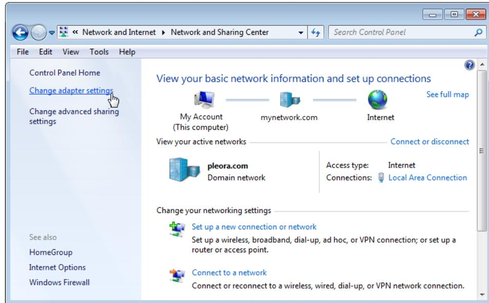
4. Configure the NIC for jumbo packets (more often referred to as jumbo frames) and set the NIC's **Receive Buffers (Receive Descriptors)** to the maximum available value. Using jumbo packets allows you to increase system performance. However, you must ensure your NIC and GigE switch (if applicable) support jumbo packets.
