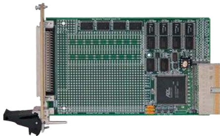
Fig. 1.11 - Typical Prototyping Module (image shown - Pickering's Breadboard Module 40-220)
